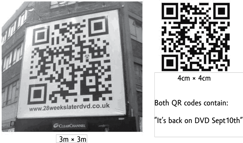
Figure 2. The variety of sizing in the design of two QR codes containing the same data
